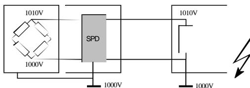
Fig.21 Systems with unavoidable multiple points of earthing should use an SPD to divert surges to a local ground. By doing so, the whole system will rise and fall at the same potential.
