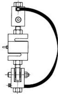
Fig. 15 Correct installation of S-type load cell.
