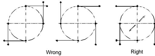
Fig.13 Placing rods as indicated in the left drawings will cause high stresses in the stay rods or rotation of the vessel.
