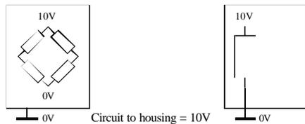
Fig.19 Load cell and indicator are both connected to a separate earth, at a considerable distance from each other.
