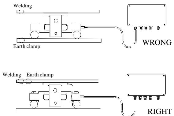
through the load cells. Furthermore, connect a flexible copper lead over each load cell.
