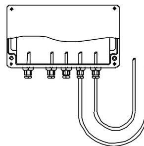
Fig.16 Correct installation of junction box; cable entries downwards and dripping loops.
