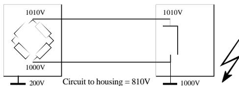
Fig.20 The potential at the earthing points will rise as a direct result of a lightning strike (to earth). However, both points will not rise to the same potential because of the ground resistance. Although the excitation voltage remains 10V, the potential difference between circuit and housing increases far above an acceptable value.
