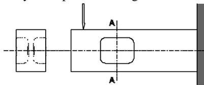
Fig.3 Principle of shear-web sensing element
