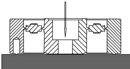
The geometrical design of the sensing element provides enhanced specifications in terms of creep and hysteresis compared to shear and bending as a measuring principle.
