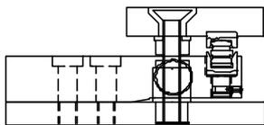
Fig.12 Self aligning mount, based on a rocker pin load introduction. The top plate is held captive to provide lift-off protection and to restrict the horizontal movement.
