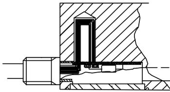
Fig.10 Water block cable entry
