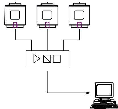
cell is used then it is possible to sample the load cells simultaneously. The junction box is then connected to a host controller via a standard interface.
