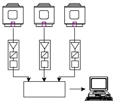
Fig.5: Electronics built in the load cell cable
