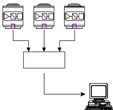
Fig.6: Digital load cell system
